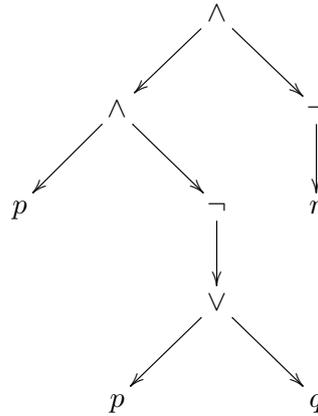
Using priority, this formula can be written with fewer parentheses:  $p \wedge \neg(p \vee q) \wedge \neg r$  using logical notation,  $p \overline{p+q} \bar{r}$  using boolean notation. Similarly, give the tree representation, logical notation and boolean notation, both using as few parentheses as possible of the following formulas:
